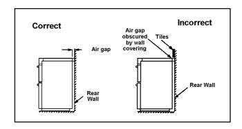
**Note:** Vapours from the oven vents may in time cause discolouration of wallcoverings behind the appliance. For ease of cleaning it may be preferable to tile behind the appliance.
